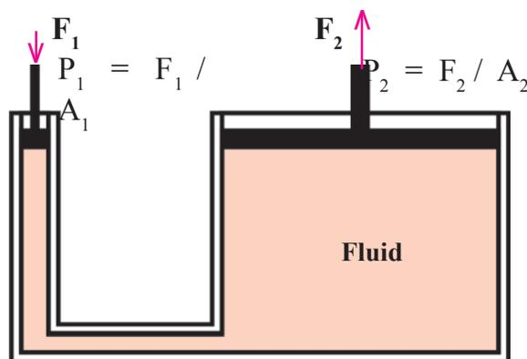
Fig-12: Application of Pascal's principle (bramah press)
