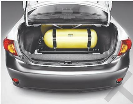
*Fig - 2: CNG cylinder in a car*
