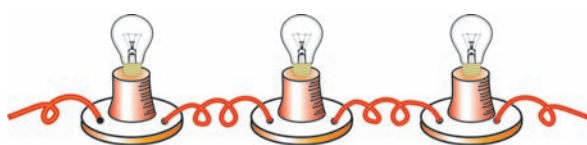
Fig. 12 - Bulbs connected in series
