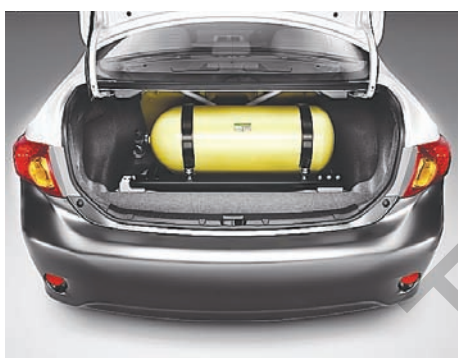
Fig - 2: CNG cylinder in a Car
