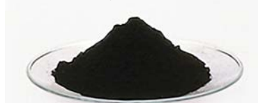
fig-15(a): Copper Oxide change into black colour
