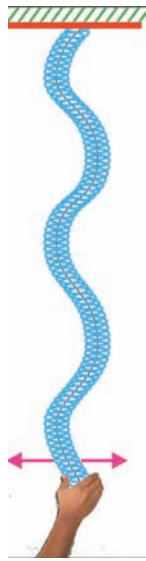
Fig-5: Transverse waves in a slinky
