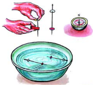
Fig-2: Making needle magnets and floating them in a bowl of water.
