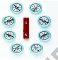
Fig-1(b) Change in direction of the needle of the compass due to bar magnet.
